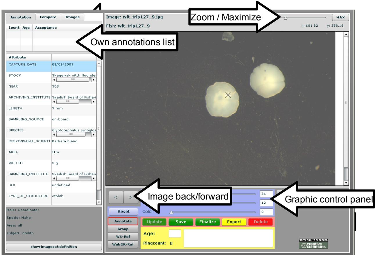
Figure 5: The annotation interface with explanations
