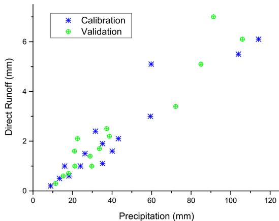
Figure 2. Measured direct runoff depth plotted as a function of precipitation depth for the 30 events used for the calibration and the validation of the model
