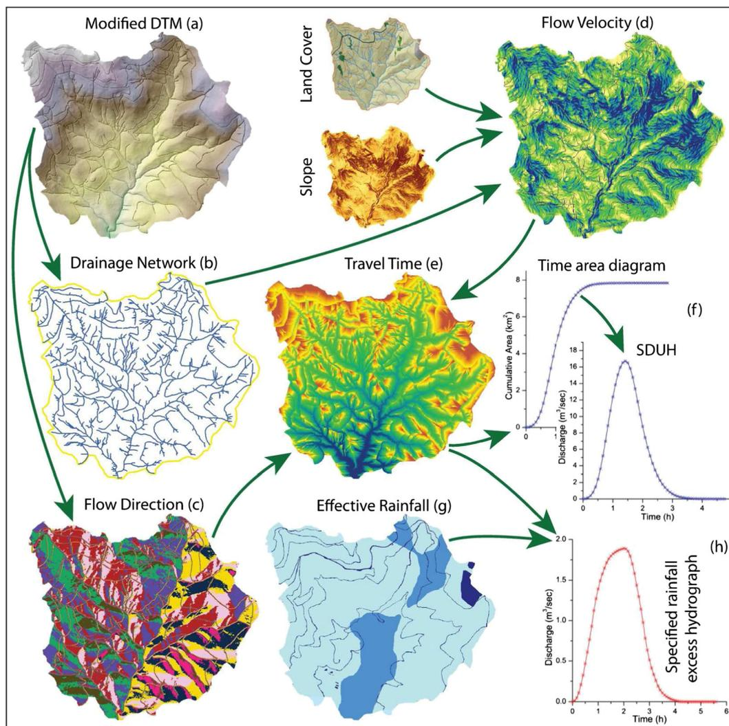
Figure 4. Graphical representation of the required steps for the determination of the SDUH using GIS
