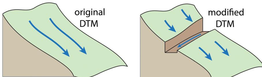
Figure 3. DTM modification to reflect the effect of roads on runoff routing
