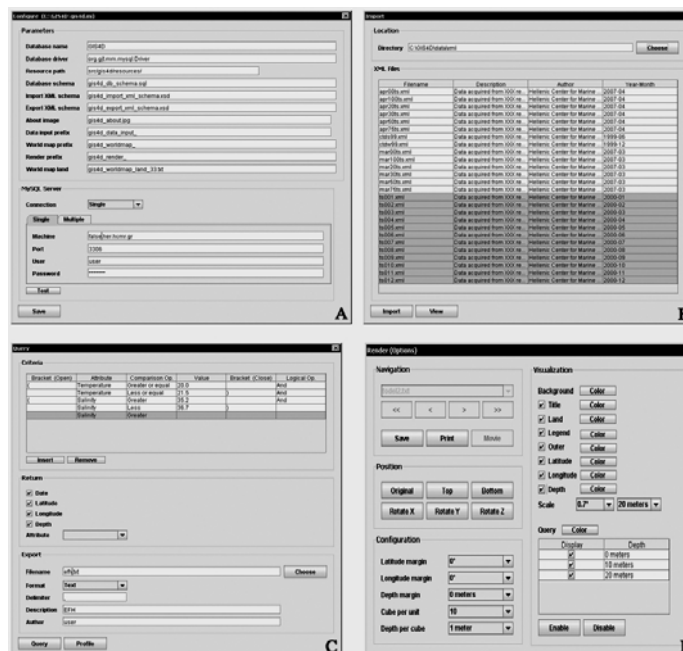
Fig. D8-13b. Fig. 2. The four main user interface menus of the JAVA tool: Configuration of single or multiple data servers (A), import of multiple XML-formatted data files (B), 3D query with multiple variables and range values of interest (C), and rendering-visualization capabilities (D).
