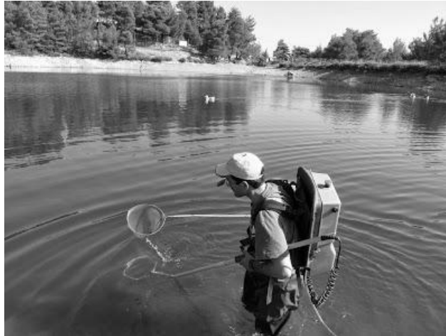
Fig. 10. Sampling with a back-pack electrofisher along the shore of a small lake can only be a “qualitative form” of sampling since reaching larger-sized fishes, and some deeper-water inhabitants is usually not possible. In this clear-water reservoir fish are stunned and collected only where they may seek cover or by surprise. Source: HCMR WFD monitoring (Photo: I. Karaouzas, Lake Beletsi, Attika).
