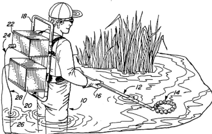
Fig. 5. Typical battery powered backpack electrofishing set up. [Figure adapted from U.S. Pat. No. 5,214,873: Electrofishing pole.]
