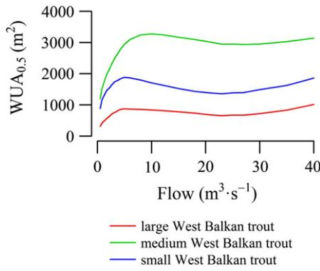
**Fig. 5.** Curves relating WUA<sub>0.5</sub> and stream flow within a range of summer flows which are possible to occur under all the examined scenarios for three size classes of W. B. trout.
