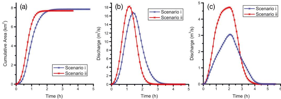
Figure 7. Time–area diagrams (a), spatially distributed unit hydrograph (b) and direct runoff hydrograph (c), for the two scenarios examined
