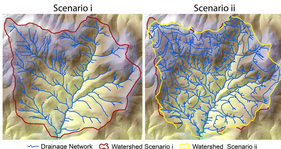
Figure 6. Effects of roads on the water divide and the drainage network
