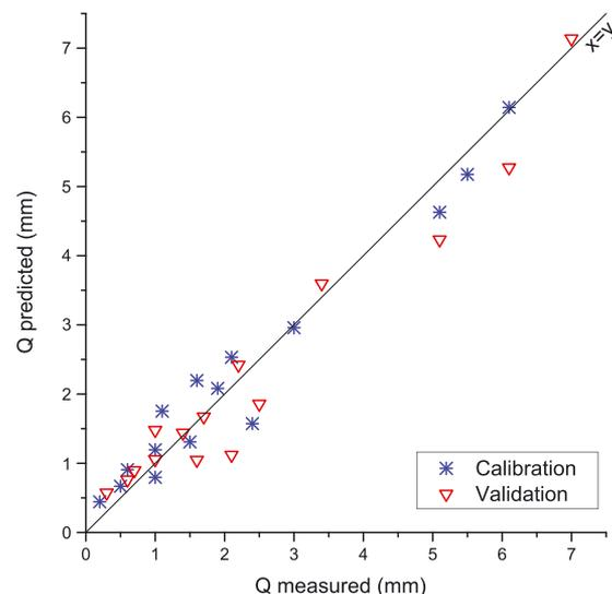
Figure 5. Comparison between the predicted and the measured direct runoff volumes for both the calibration and the validation phases
