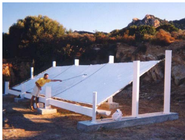
FIGURE 20 Inclined fog collector (top) (Khamdevi & Matius 2023) and funnel-shaped dew collector (bottom) (Beysens et al., 2013)
